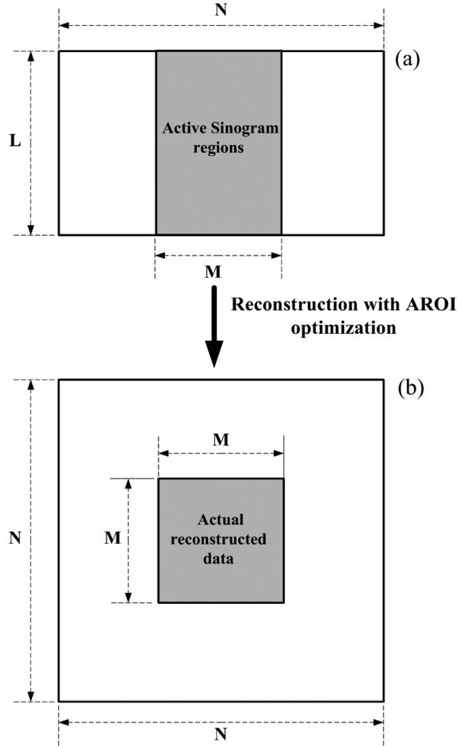
Fig. 1. Schematic diagram of FBP reconstruction algorithm with the AROI method: (a) the scale of Sinogram; (b) the scale of reconstructed image;  $N$  is the number of the linear array X-ray detector elements;  $L$  is the number of rotation angles; and  $M$  is the number of available detector elements with the AROI method.
