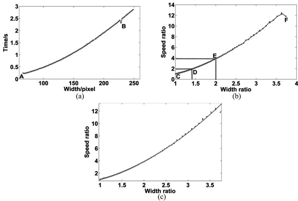
Fig. 7. Reconstruction speed. (a) Relationship between the reconstruction time and the width of the projection image with the AROI method; (b) relationship between the speed ratio and the width ratio of the projection image; (c) curve fitting of the relationship between speed ratio and width ratio. The speed ratio is the time required by the original method divided by the time required by the AROI method. Similarly, the width ratio is the detector width divided by the ROI width.
