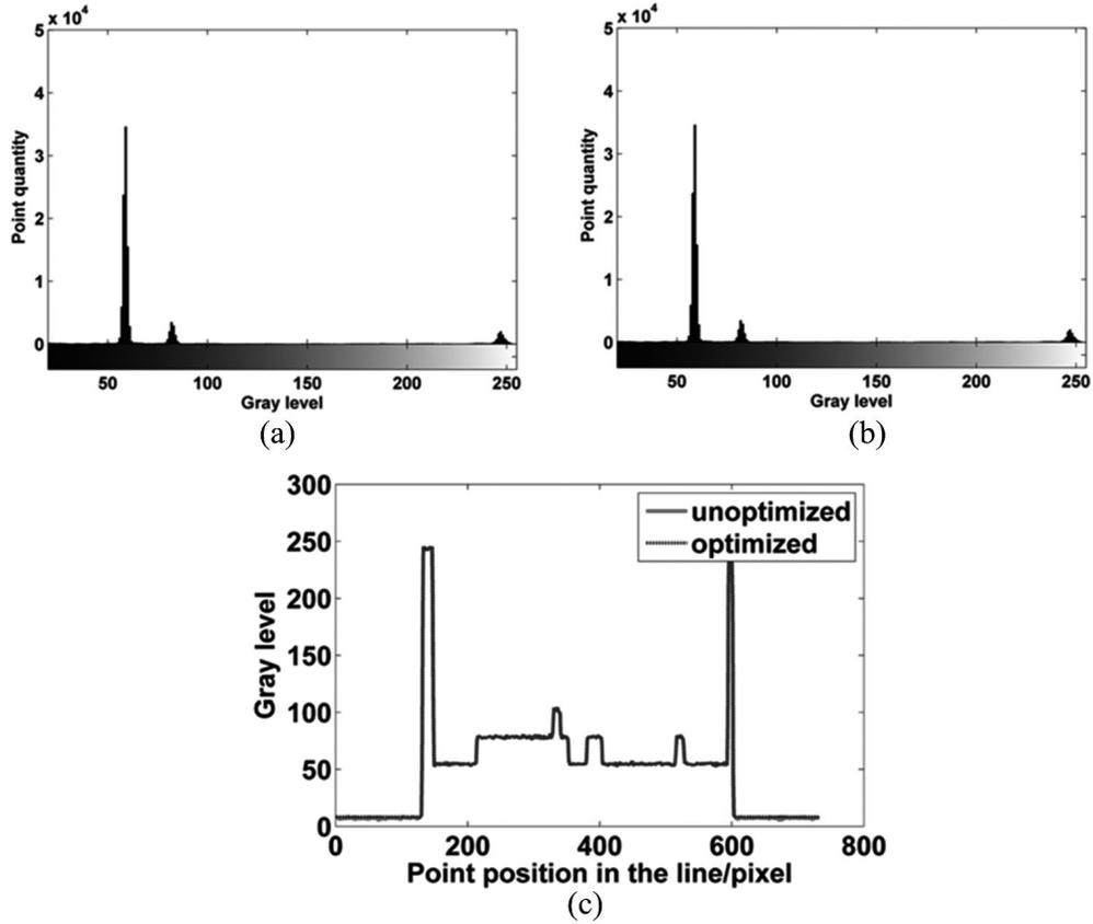
Fig. 5. Comparison of the reconstruction quality of two methods using the Shepp-Logan model. (a) Gray histogram of Fig. 4(b); (b) gray histogram of Fig. 4(c); (c) gray-scale distribution curve of the white lines in Fig. 4(a) and Fig. 4(b). The gray levels in Fig. 5(a) and Fig. 5(b) range from 20 to 255.
