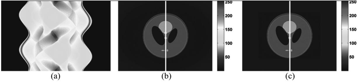
Fig. 4. Shepp-Logan model reconstruction: (a) projection data of the Shepp-Logan model; (b) reconstruction image without AROI optimization; (c) reconstruction image with AROI optimization.
