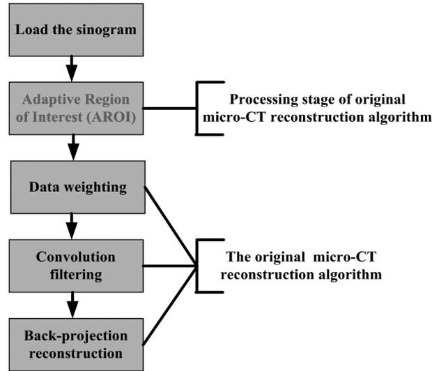
Fig. 2. Flowchart of micro-CT reconstruction algorithm with the AROI method.
