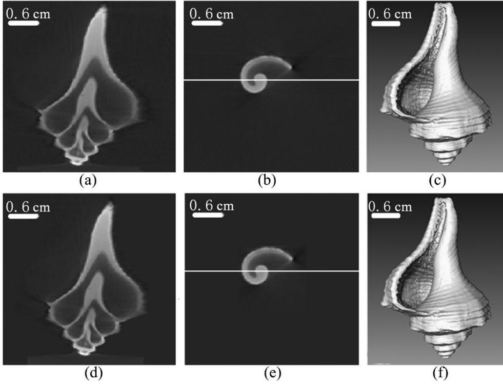
Fig. 8. Reconstruction image of the conch sample. (a), (b), and (c) are the reconstruction images without the AROI method. (d), (e), and (f) are the optimized reconstruction images with the AROI method. (a) and (d) are slice reconstruction images of the y-z plane; (b) and (e) are slice reconstruction images of the x-y plane; (c) and (f) are the 3D reconstruction images.
