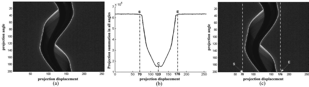
Fig. 3. Steps of AROI: (a) conch slice projection data with a cone-beam micro-CT; (b) dimension reduction for searching  $S$  point and  $E$  point; (c) the edge of the actual object data as shown by white dashed lines.
