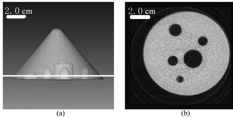
Fig. 6. The conical model reconstruction: (a) 3D reconstruction of the cone; (b) a slice reconstruction image of the white line in Fig. 6(a).
